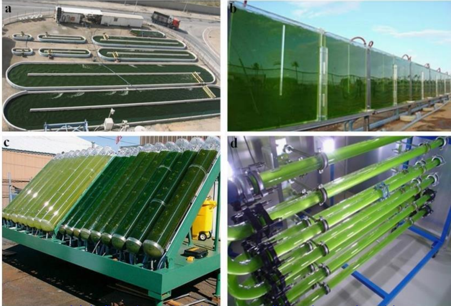
Raceway pond (a), flat-plate photobioreactor (b), column photobioreactor (c) and tubular photobioreactor (d)
