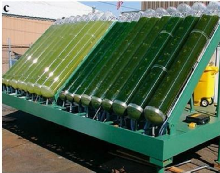
Raceway pond (a), flat-plate photobioreactor (b), column photobioreactor (c) and tubular photobioreactor (d)
