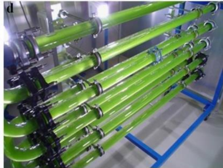
Raceway pond (a), flat-plate photobioreactor (b), column photobioreactor (c) and tubular photobioreactor (d)
