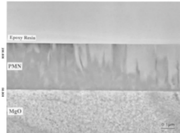
Figure 6.12. Cross-sectional TEM image of sputtered PMN thin films epitaxially grown onto (001) MgO.
