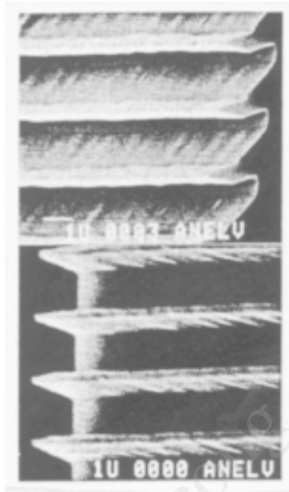
Figure 7.12. Typical vertical structures of \text{SiO}_2 on Si, etched by an ECR ion-beam system. (Courtesy of Anelva.)
