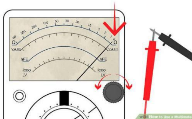
Picture 1.4. Adjusting Zero point
