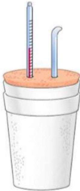
▲ FIGURE 7-6 A Styrofoam "coffee-cup" calorimeter
