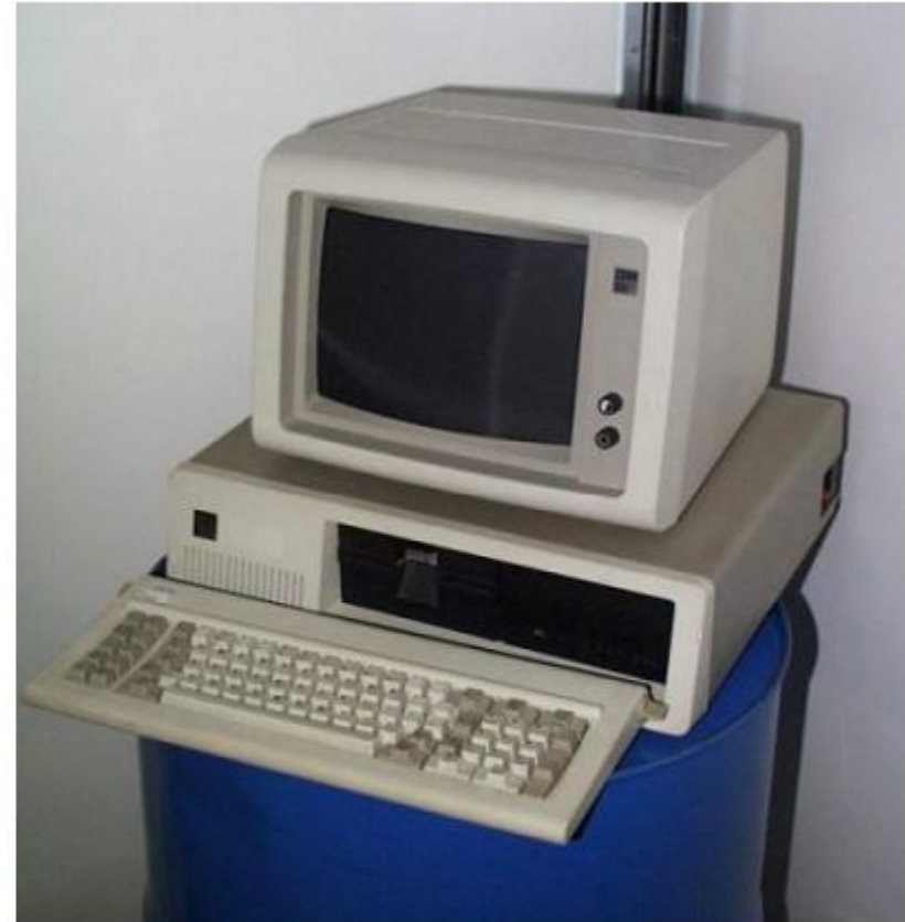
XT computer with Intel 8086 chip
