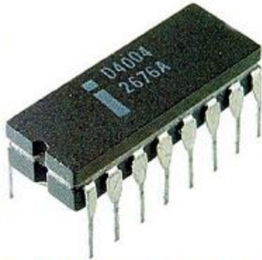
Intel 4004 with 2300 transistors inside
