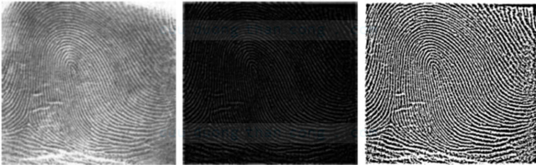
a b c (a) Thumb print. (b) Result of highpass filtering (a). (c) Result of thresholding (b).
