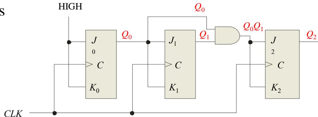
The next slide shows how to analyze this counter by writing the logic equations for each input. Notice the inputs to each flip-flop...
