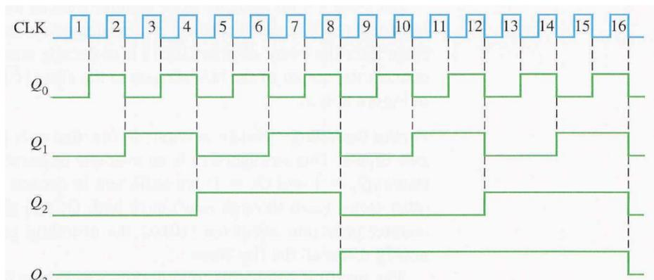
Asynchronous counters are sometimes called **ripple** counters
