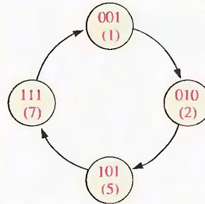
**Solution Step 1:** The state diagram is as shown. Although there are only four states, a 3-bit counter is required to implement this sequence because the maximum binary count is seven. Since the required sequence does not include all the possible binary states, the invalid states (0, 3, 4, and 6) can be treated as “don’t cares” in the design. However, if the counter should erroneously get into an invalid state, you must make sure that it goes back to a valid state.
