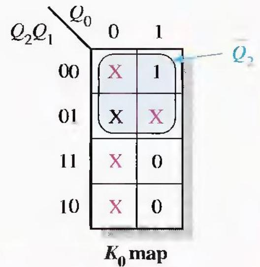
**Step 5:** Group the 1s, taking advantage of as many of the “don’t care” states as possible for maximum simplification, as shown in Figure 8–33. Notice that when *all* cells in a map are grouped, the expression is simply equal to 1. The expression for each  $J$  and  $K$  input taken from the maps is as follows:
