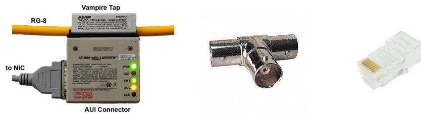
Tap, T-connector, and RJ-45
