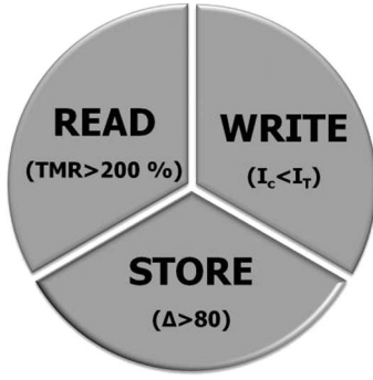
Fig. 14. An example STT-MRAM trilemma. Simultaneously three properties have to be satisfied: reading, writing, and storing. In this example, it is necessary to have TMR > 200% for reliable reading, switching current less than that supplied by a small transistor for small cell size, and thermal stability factor \Delta > 80 to meet a desired data retention goal.
