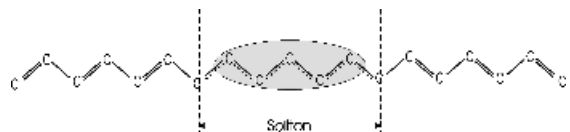
Figure 13.24 A soliton in trans -polyacetylene. The shaded ellipse in the centre of the soliton may represent either an electron hole (creating a positively charged soliton), a single electron (creating a neutral soliton) or two electrons (creating a negative soliton)
