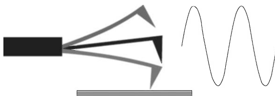
Figure 5.14 The tapping mode. The oscillation of the cantilever is dampened when the tip touches the sample surface at each cycle. The image is formed by keeping the oscillation amplitude constant. (Reproduced with permission from Ref. [3]. © 2004 Humana Press.)
