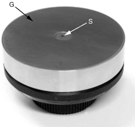
Figure 3.8 Hand-grinding jig for TEM specimen preparation. A disc (S) is glued to the center of the jig and the guide ring (G) controls the amount of grinding.
