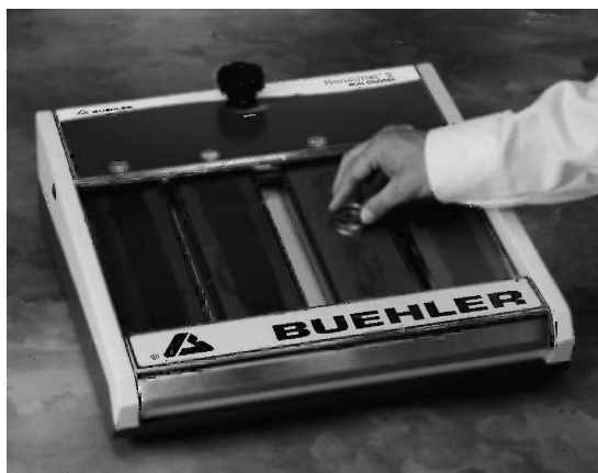
Figure 1.21 Hand grinding using a simple hand grinding device. (Reproduced with permission of Buehler Ltd.)
