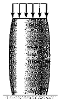
Compression causes material to bulge out (b)
