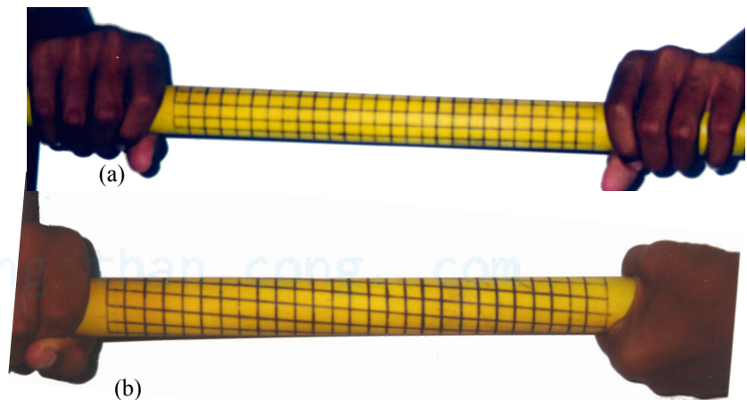
Figure 5.16 Torsional deformation: (a) original grid; (b) deformed grid. (Courtesy of Professor J. B. Ligon.)
