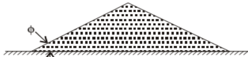
Fig. 1.4.2. Heap created by a free flowing material
