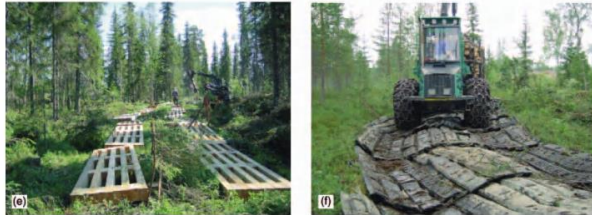
Figure 7 Illustration of (a) site damage by excessive rutting in cases of long extraction routes, and (b) laying of brash mat to minimize damage, and (c) machine band tracks and (d) wheel chains for enhancement of flotation and traction, respectively. Other possible mechanical strengthening of ground with (e) wooden platforms and (f) discarded fire mats may be applied, but the economic feasibility is a function of distance to be strengthened and volume of wood to be transported. Reproduced with permission from Forest Engineering Unit, University College Dublin; Clark Forestry Equipment UK; and Department of Forest Resource Management, University of Helsinki, respectively.
