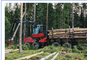
Figure 8 A Combi-machine or HarWader for combined harvesting and extraction. Reproduced with permission from Partek Forest, Sweden.
