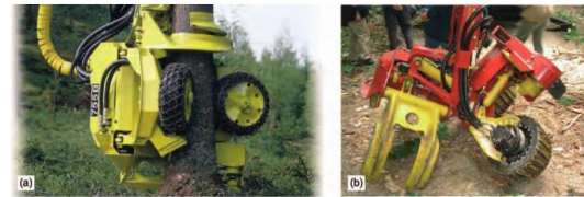
Figure 11 Single grip harvester head with (a) stem optimization capability and (b) a variance consisting of articulated delimbing knives and feed rollers for autonomous processing and loading capability. Reproduced with permission from Timberjack OY, Finland and Forest Engineering Unit, University College Dublin.
