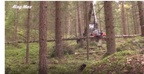
Figure 3 Full-pole method of wood harvesting. Adapted with permission from Staat KAG and Wiksten NA (1984) Tree Harvesting Techniques . Kluwer Academic Publishers, Dordrecht, The Netherlands: Martinus Nijhoff.
