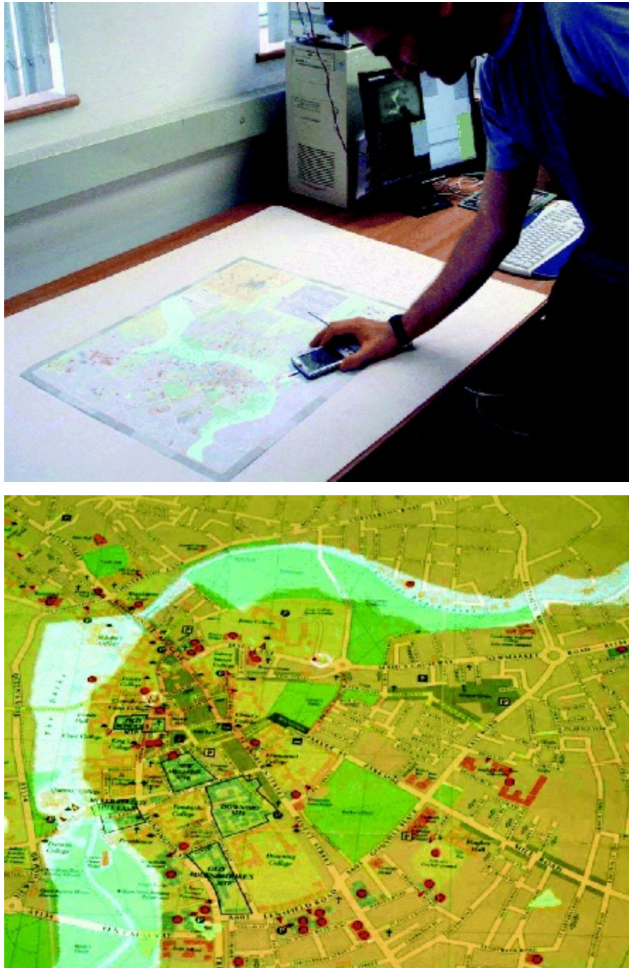
Figure 6.30 An augmented map showing the flooded areas at high water level overlaid on the paper map. The handheld device is used to interact with entities referenced on the map
