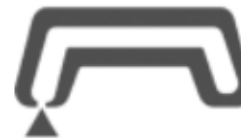
Gas-Assisted Injection Molding (GAIM).
