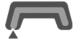
Water-Assisted Injection Molding (WAIM).
