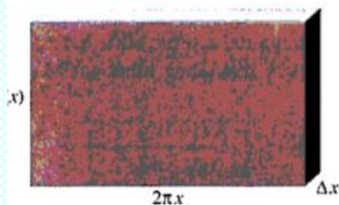
c. The "unwrapped" flattened shell has volume \Delta V = 2\pi x f(x) \Delta x
