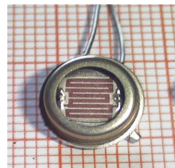
Light dependent resistor (LDR)
