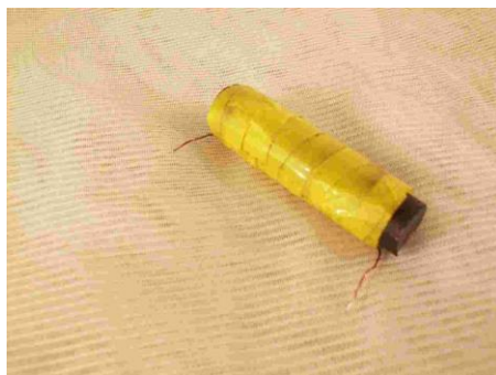
Ferrite Rod Inductor
