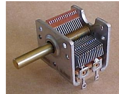
Tuning/Air Variable Capacitor
