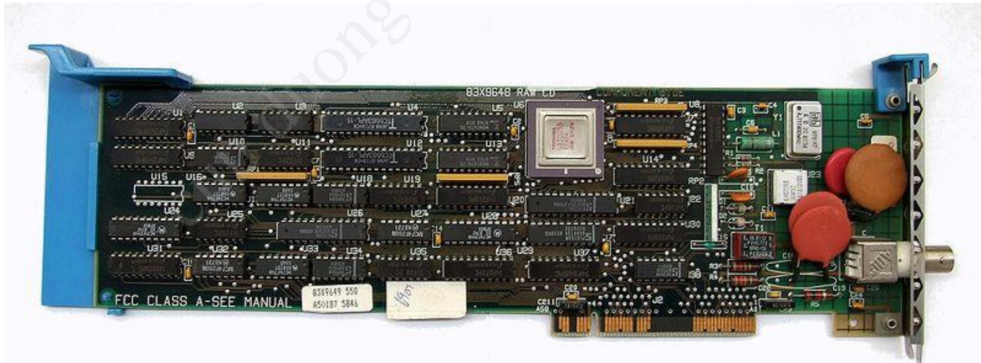
Network Interface Card IBM 83X9648 (MCA)
