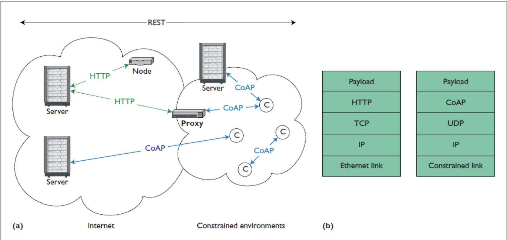
Implementing the Web architecture with HTTP and the Constrained Application Protocol (CoAP). (a) HTTP and CoAP work together across constrained and traditional Internet environments; (b) the CoAP protocol stack is similar to, but less complex than, the HTTP protocol stack.
