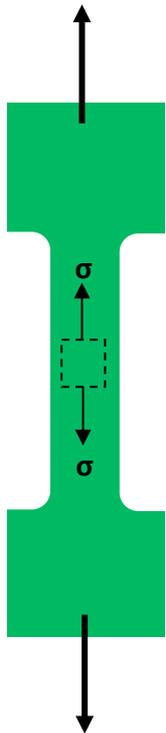
Consider the simple tension with a sample subjected to tension in the  $x$ -direction. The state of stress is represented by the one-dimensional field
