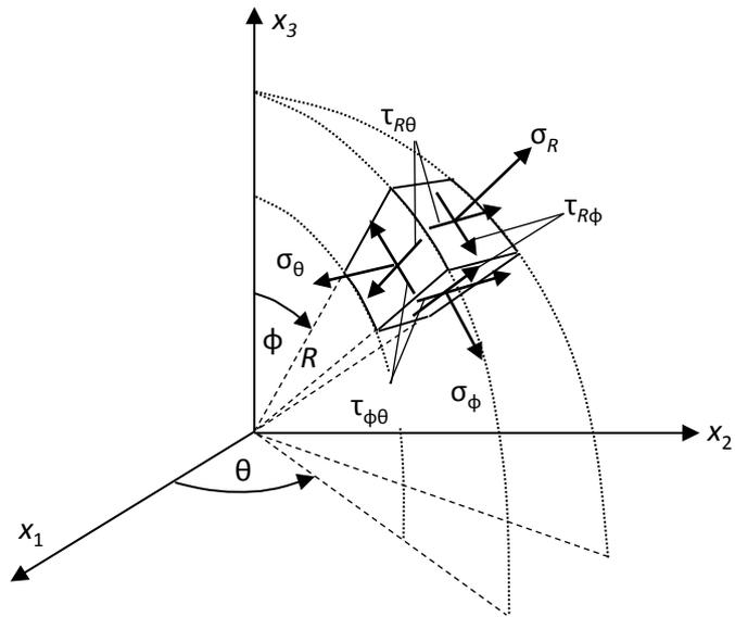
$$\boldsymbol{\sigma} = \begin{bmatrix} \sigma_R & \tau_{R\phi} & \tau_{R\theta} \\ \tau_{R\phi} & \sigma_\phi & \tau_{\phi\theta} \\ \tau_{R\theta} & \tau_{\phi\theta} & \sigma_\theta \end{bmatrix}$$
