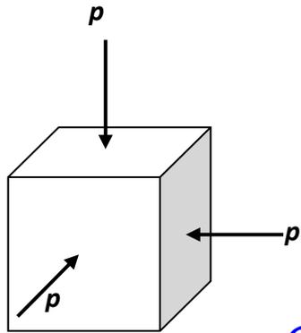
The final example is associated with the uniform compression (or tension) loading of a cubical specimen. This type of test can be realizable if the sample was placed in a high-pressure compression chamber. The state of stress for this case is given by
