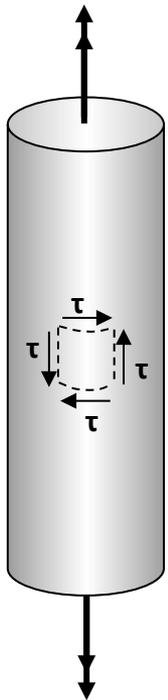
If a thin-walled cylinder is subjected to torsion loading, the state of stress on the surface of the cylindrical sample is given by
