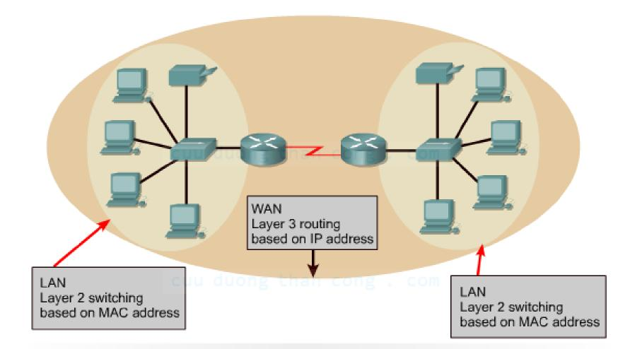
Layer 2 switching takes place within the LAN. Layer 3 routing moves traffic between broadcast domains. This requires the hierarchical addressing format that a Layer 3 addressing scheme like IP provides.
