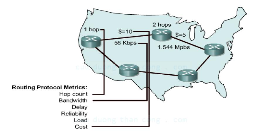
Routing metrics are values used in determining the advantage of one route over another, which used by router.
