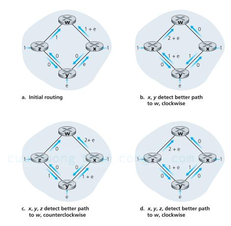
Figure 4.29 ♦ Oscillations with congestion-sensitive routing
