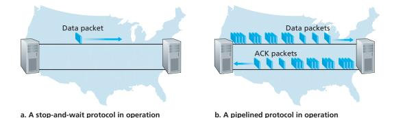
Figure 3.17 ♦ Stop-and-wait versus pipelined protocol
