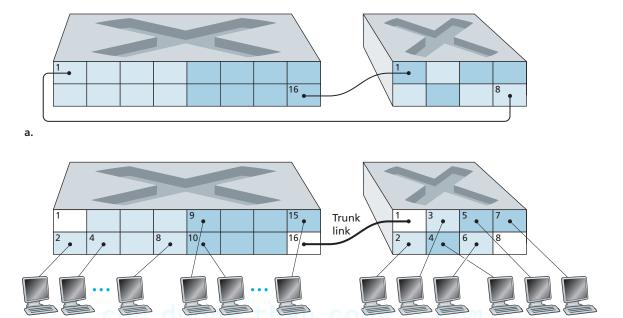
Figure 5.26 ♦ Connecting two VLAN switches with two VLANs: (a) two cables (b) trunked
