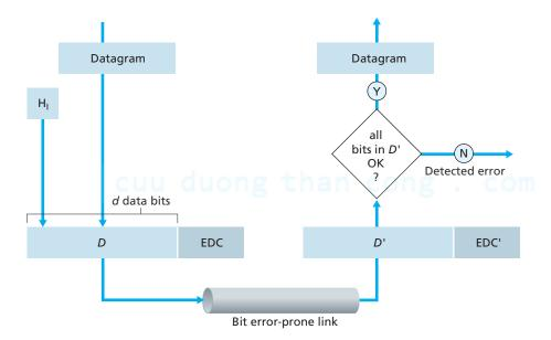
Figure 5.3 ◆ Error-detection and -correction scenario
