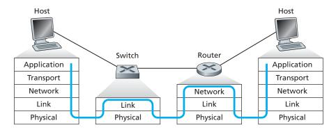
Figure 5.24 ◆ Packet processing in switches, routers, and hosts
