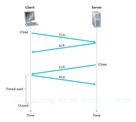
Figure 3.40 ♦ Closing a TCP connection
