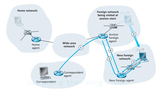
Figure 6.26 ♦ Mobile transfer between networks with direct routing
