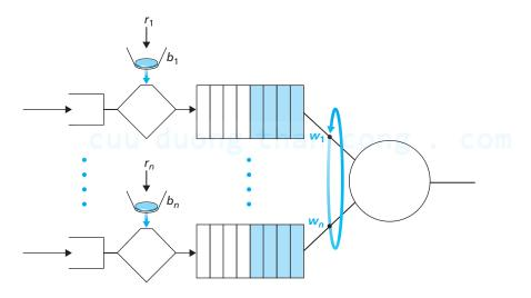
**Figure 7.24 ♦** *n* multiplexed leaky bucket flows with WFQ scheduling
