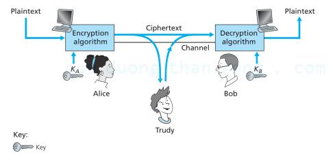
Figure 8.2 ◆ Cryptographic components
