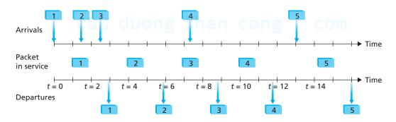
Figure 7.18 ◆ The FIFO queue in operation
