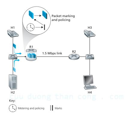
Figure 7.15 ♦ Policing (and marking) the audio and HTTP traffic classes
