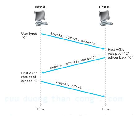
Figure 3.31 ◆ Sequence and acknowledgment numbers for a simple Telnet application over TCP
