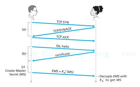
Figure 8.25 ♦ The almost-SSL handshake, beginning with a TCP connection
