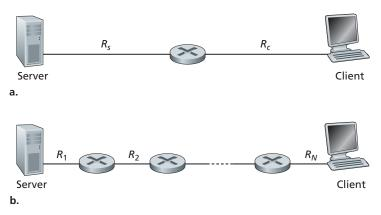
Figure 1.19 ♦ Throughput for a file transfer from server to client
