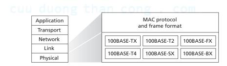
Figure 5.21 ◆ 100 Mbps Ethernet standards: a common link layer, different physical layers
