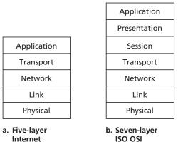
Figure 1.23 ♦ The Internet protocol stack (a) and OSI reference model (b)
