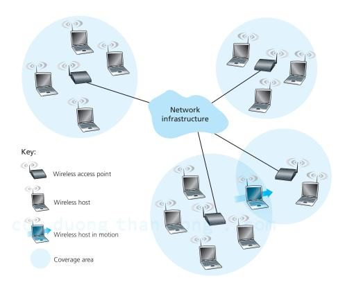
Figure 6.1 ◆ Elements of a wireless network
