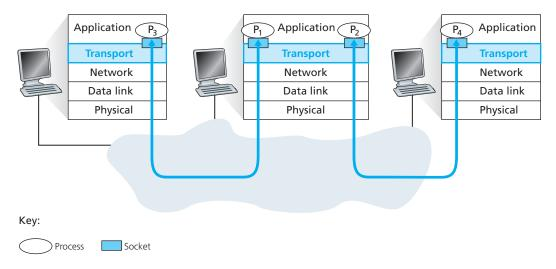
Figure 3.2 ◆ Transport-layer multiplexing and demultiplexing
