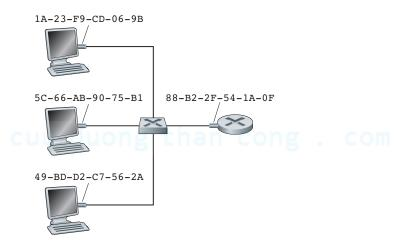
Figure 5.16 ♦ Each interface connected to a LAN has a unique MAC address
