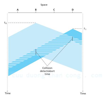
Figure 5.13 ◆ CSMA with collision detection
