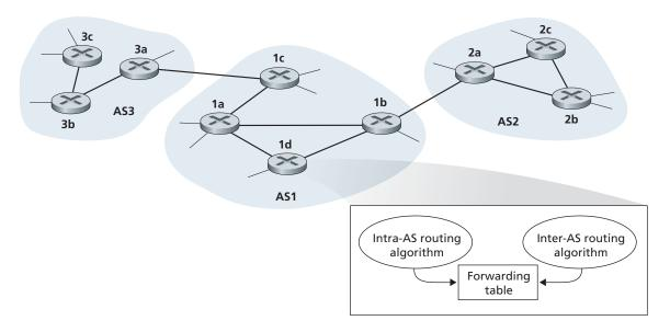
Figure 4.32 ♦ An example of interconnected autonomous systems
