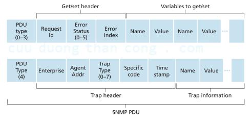
Figure 9.4 ♦ SNMP PDU format
