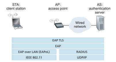
Figure 8.32 ◆ EAP is an end-to-end protocol. EAP messages are encapsulated using EAPoL over the wireless link between the client and the access point, and using RADIUS over UDP/IP between the access point and the authentication server
