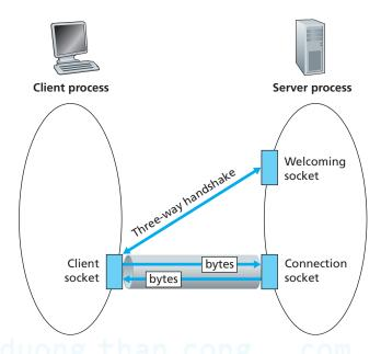
Figure 2.29 ♦ The TCPServer process has two sockets
