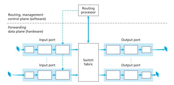
Figure 4.6 ♦ Router architecture
