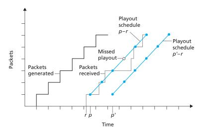
Figure 7.7 ♦ Packet loss for different fixed playout delays
