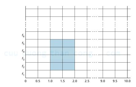
Figure 6.20 • Twenty 0.5 ms slots organized into 10 ms frames at each frequency. An eight-slot allocation is shown shaded.
