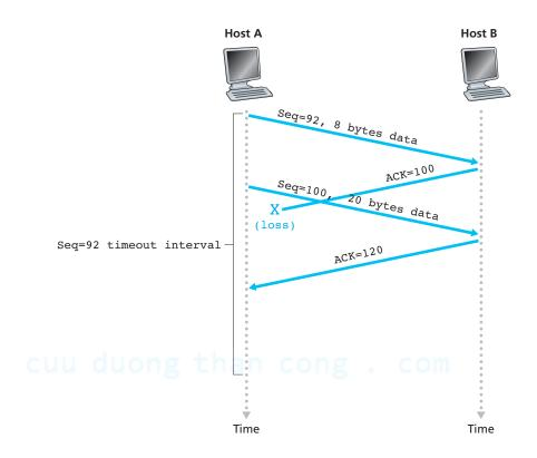
Figure 3.36 ♦ A cumulative acknowledgment avoids retransmission of the first segment
