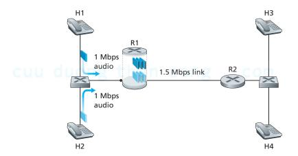
Figure 7.27 ♦ Two competing audio applications overloading the R1-to-R2 link
