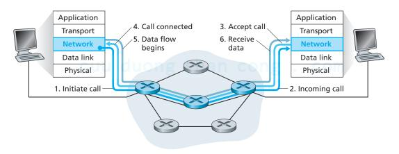
Figure 4.4 ♦ Virtual-circuit setup
