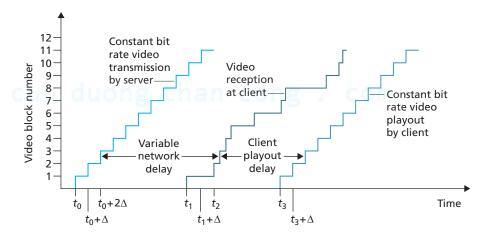
Figure 7.1 ♦ Client playout delay in video streaming
