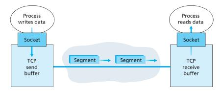
Figure 3.28 ♦ TCP send and receive buffers
