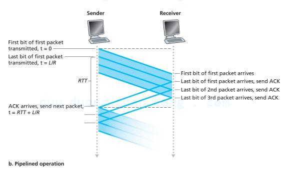
Figure 3.18 • Stop-and-wait and pipelined sending
