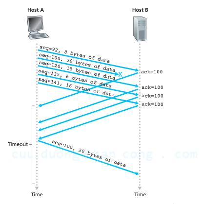
Figure 3.37 ♦ Fast retransmit: retransmitting the missing segment before the segment's timer expires
