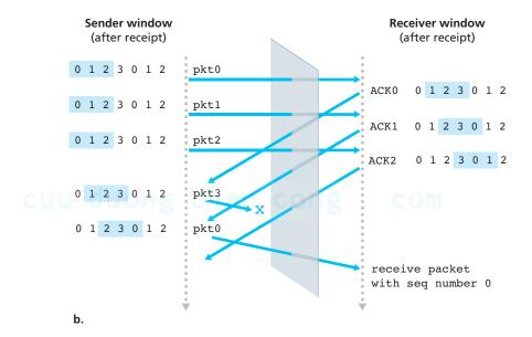
Figure 3.27 ♦ SR receiver dilemma with too-large windows: A new packet or a retransmission?
