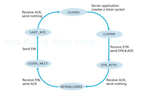
Figure 3.42 ♦ A typical sequence of TCP states visited by a server-side TCP
