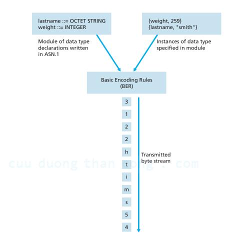
Figure 9.9 ♦ BER encoding example
