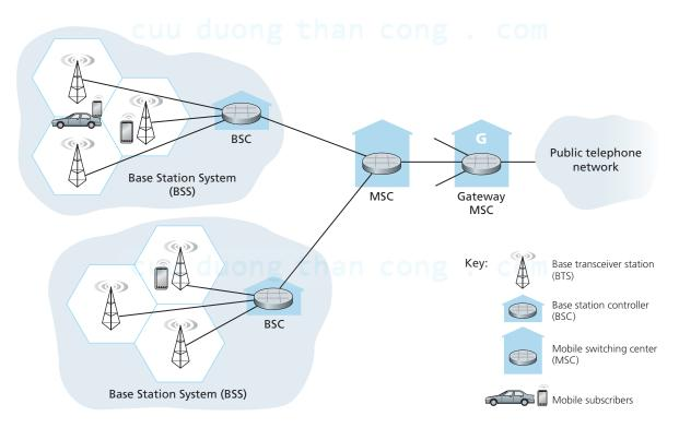
Figure 6.18 ♦ Components of the GSM 2G cellular network architecture
