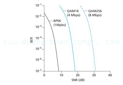
Figure 6.3 ♦ Bit error rate, transmission rate, and SNR
