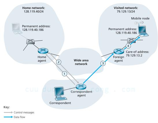
Figure 6.25 ♦ Direct routing to a mobile user
