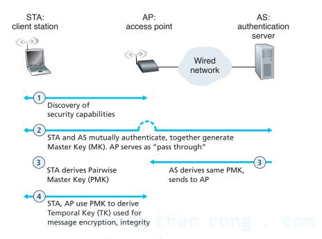
**Figure 8.31 ♦** 802.11i: four phases of operation
