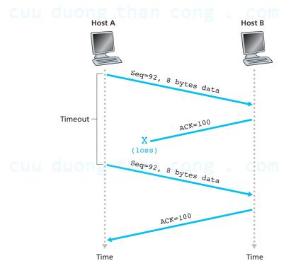
Figure 3.34 ◆ Retransmission due to a lost acknowledgment
