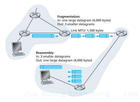
Figure 4.14 ◆ IP fragmentation and reassembly
