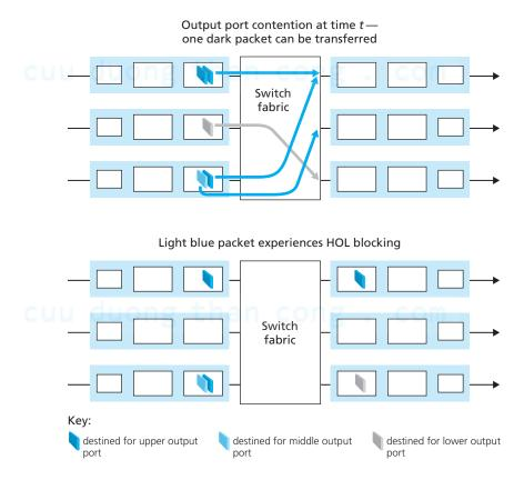
Figure 4.11 ♦ HOL blocking at an input queued switch
