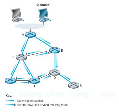
Figure 4.50 ♦ Reverse path forwarding, the multicast case
