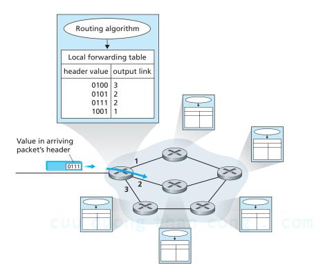
Figure 4.2 ♦ Routing algorithms determine values in forwarding tables
