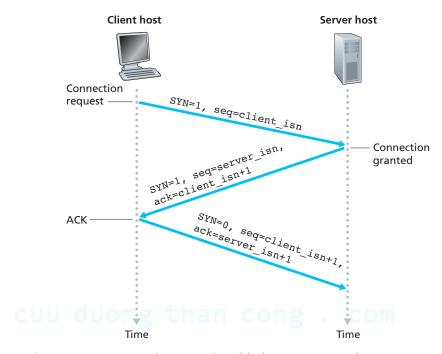
Figure 3.39 ♦ TCP three-way handshake: segment exchange
