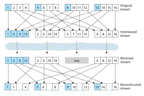
Figure 7.9 ◆ Sending interleaved audio
