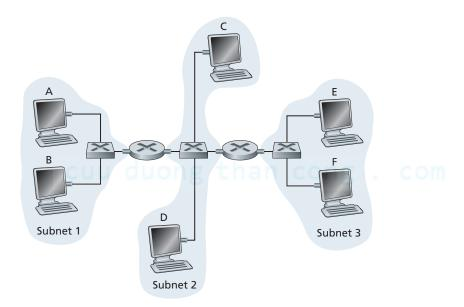
Figure 5.33 ♦ Three subnets, interconnected by routers
