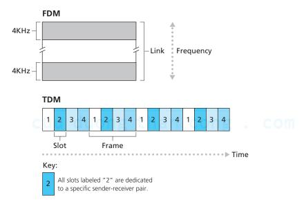
Figure 1.14 • With FDM, each circuit continuously gets a fraction of the bandwidth. With TDM, each circuit gets all of the bandwidth periodically during brief intervals of time (that is, during slots)
