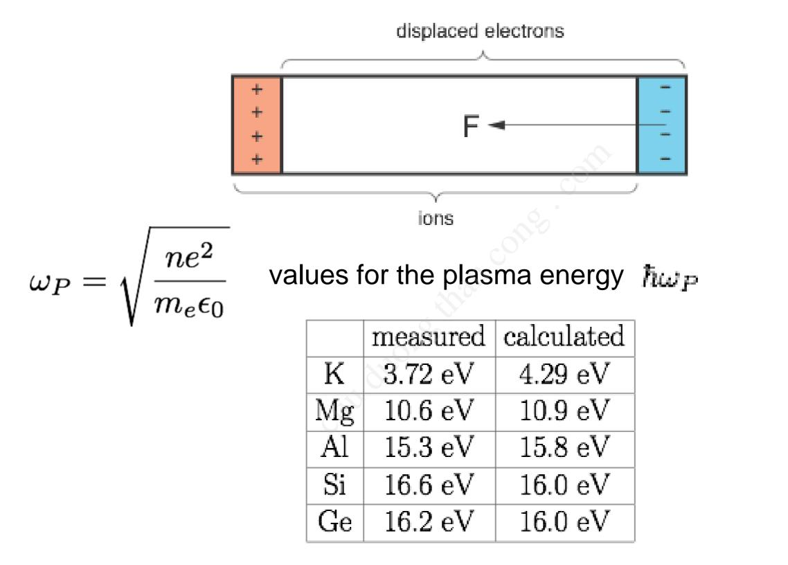
Iongitudinal collective mode of the whole electron gas
