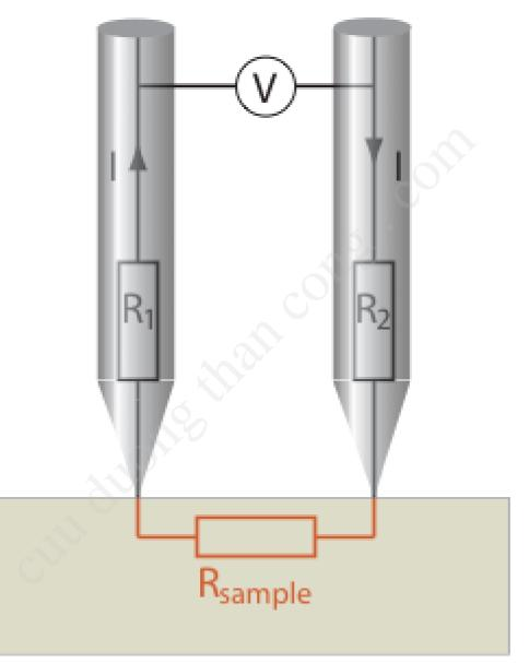
A two-point probe can be used but the contact or wire resistance can be a problem, especially if the sample has a small resistivity.
