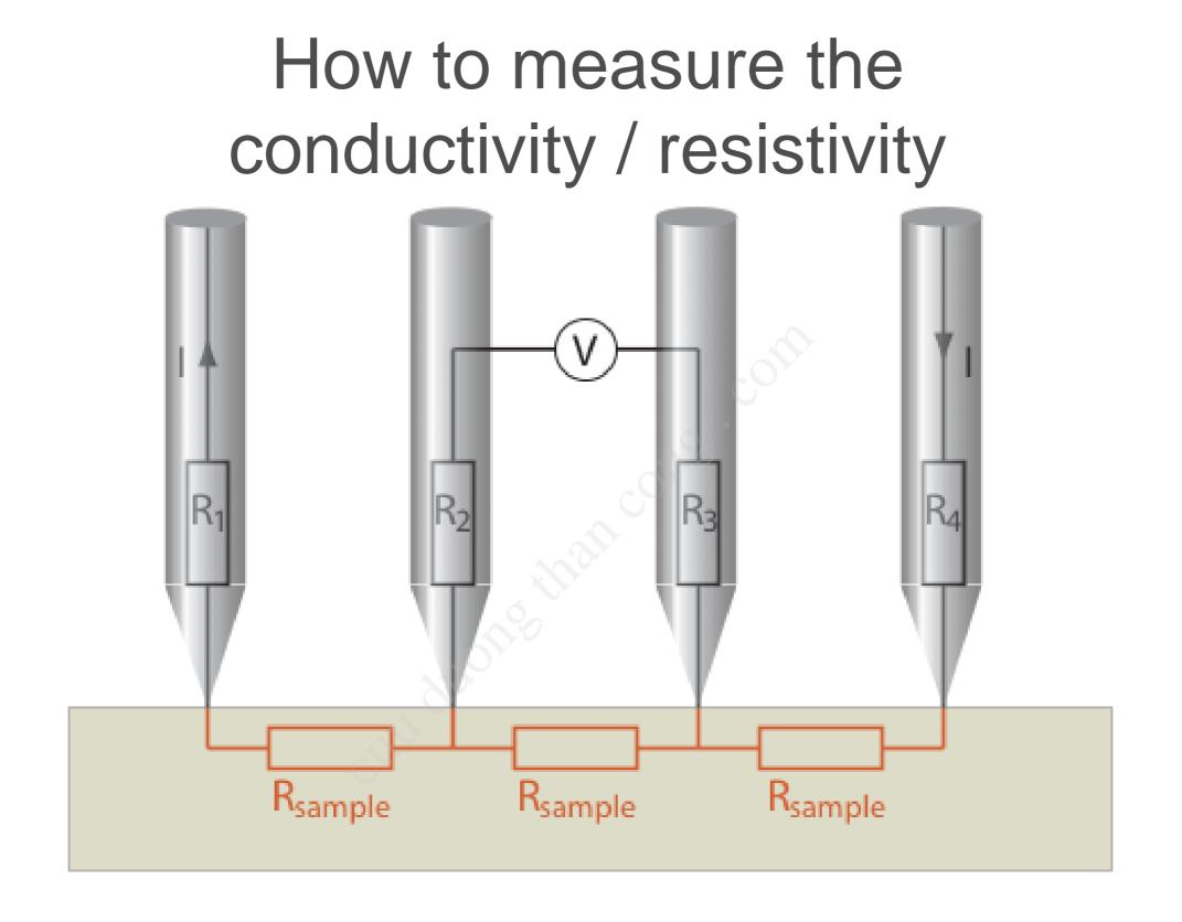
The problem of contact resistance can be overcome by using a four point probe.
