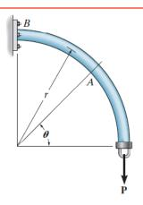
**1–30.** A differential element taken from a curved bar is shown in the figure. Show that  $dN/d\theta = V$ ,  $dV/d\theta = -N$ ,  $dM/d\theta = -T$ , and  $dT/d\theta = M$ .
