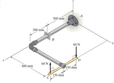
\*1–28. The brace and drill bit is used to drill a hole at O. If the drill bit jams when the brace is subjected to the forces shown, determine the resultant internal loadings acting on the cross section of the drill bit at A.
