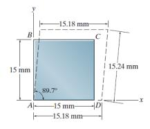
**2–23.** A square piece of material is deformed into the dashed parallelogram. Determine the average normal strain that occurs along the diagonals AC and BD.
