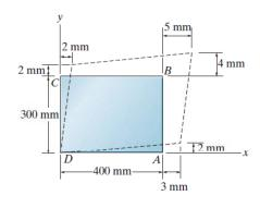
**2–19.** The piece of plastic is originally rectangular. Determine the shear strain  $\gamma_{xy}$  at corners D and C if the plastic distorts as shown by the dashed lines.
