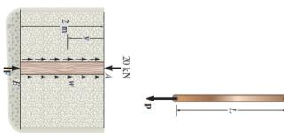
**4–14.** The post is made of Douglas fir and has a diameter of 60 mm. If it is subjected to the load of 20 kN and the soil provides a frictional resistance that is uniformly distributed along its sides of w = 4 kN/m, determine the force F at its bottom needed for equilibrium. Also, what is the displacement of the top of the post A with respect to its bottom B? Neglect the weight of the post.
