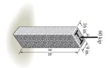
of 8 ft. How far does the column shorten? It has an original length the force is shared equally between the steel and concrete. the column, determine the required area of the steel so that concrete as shown. If an axial force of 60 kip is applied to The A-36 steel column is encased in high-strength
