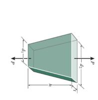
4-25. Determine the elongation of the A-36 steel member when it is subjected to an axial force of 30 kN. The member is 10 mm thick. Use the result of Prob. 4-24.
