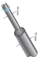
**5–122.** The built-up shaft is designed to rotate at 540 rpm. If the radius of the fillet weld connecting the shafts is r = 7.20 mm, and the allowable shear stress for the material is  $\tau_{\rm allow} = 55$  MPa, determine the maximum power the shaft can transmit.
