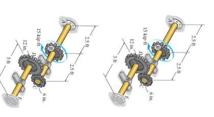
•5–89. The shafts are made of A-36 steel and have the same diameter of 4 in. If a torque of 15 kip  $\cdot$  ft is applied to gear B, determine the angle of twist of gear B.
