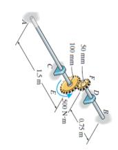
**5–87.** Determine the rotation of the gear at E in Prob. 5–86.
