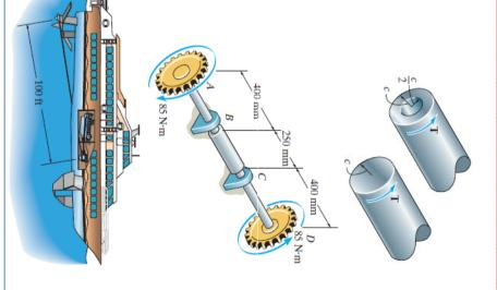
•5–49. The A-36 steel axle is made from tubes AB and CD and a solid section BC. It is supported on smooth bearings that allow it to rotate freely. If the gears, fixed to its ends, are subjected to 85-N·m torques, determine the angle of twist of gear A relative to gear D. The tubes have an outer diameter of 30 mm and an inner diameter of 20 mm. The solid section has a diameter of 40 mm.
