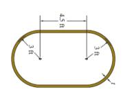
**5–114.** The mean dimensions of the cross section of an airplane fuselage are shown. If the fuselage is made from 2014-T6 aluminum alloy having an allowable shear stress of  $\tau_{\rm allow} = 18$  ksi and the angle of twist per foot length of fuselage is not allowed to exceed 0.001 rad/ft, determine the maximum allowable torque that can be sustained by the fuselage. The thickness of the wall is t = 0.25 in.
