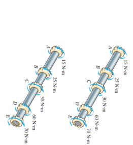
\*5–16. The solid shaft has a diameter of 40 mm. Determine the absolute maximum shear stress in the shaft and sketch the shear-stress distribution along a radial line of the shaft where the shear stress is maximum.
