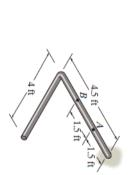
•5–17. The rod has a diameter of 1 in. and a weight of 10 lb/ft. Determine the maximum torsional stress in the rod at a section located at A due to the rod's weight.
