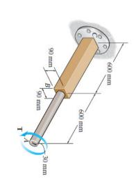
•5–101. Segments AB and BC of the shaft have circular and square cross sections, respectively. The shaft is made from A-36 steel with an allowable shear stress of  $\tau_{\rm allow} = 75$  MPa, and an angle of twist at end A which is not allowed to exceed 0.02 rad. Determine the maximum allowable torque T that can be applied at end A. The shaft is fixed at C.
