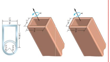
mean dimensions of the tube are shown and the tube has a thickness of 0.125 in.
