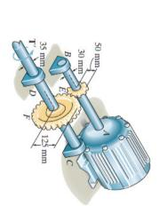
**5–14.** The solid 50-mm-diameter shaft is used to transmit the torques applied to the gears. Determine the absolute maximum shear stress in the shaft.
