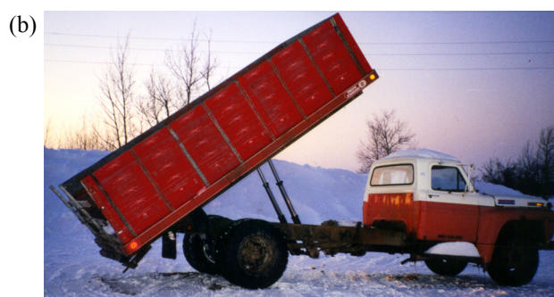
Hydraulic cylinders in a dump truck
