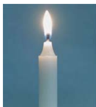
Fig. 16.4. Plumber's candle, as used by plumbers in the nineteenth century to melt lead solder when joining water pipes.
