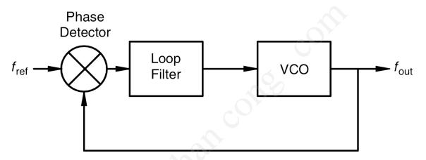
Phase detectors: If the two input frequencies are exactly the same, the phase detector output is the phase difference between the two inputs. This loop error signal is filtered and used to control the VCO frequency. The two input signals can be represented by sine waves:
