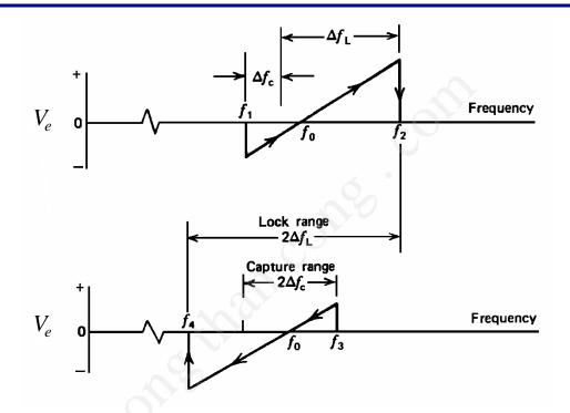
Next,  $V_e$  varies with frequency with a slope equal to the reciprocal of the VCO voltage-to-frequency conversion gain, and goes through zero as  $f = f_o$ . The loop tracks the input until the input frequency reaches  $f_2$ , corresponding to the upper edge of the lock range. The PLL then loses lock, and the error voltage drops to zero.
