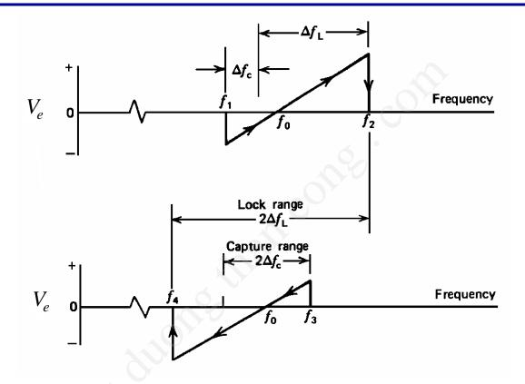
In the upper part of the above figure, the loop frequency is being gradually increased. The loop does not respond to the signal until it reaches a frequency  $f_1$ , corresponding to the lower edge of the capture range. Then, the loop suddenly locks on the input, causing a negative jump of the loop-error voltage.
