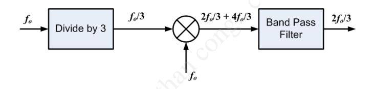
One of the most critical consideration is that the direct synthesis method requires highly selective filters. This can be reduced with the frequency synthesis method that employs a PLL.
