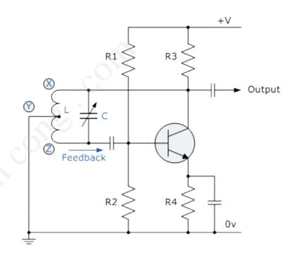
Example of <u>Hartley circuit</u> (with bias), oscillating frequency:
