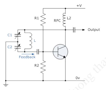
Example of <u>Colpitts circuit</u> (with bias), oscillating frequency:
