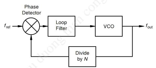
**Frequency dividers:** When the <u>output frequency</u> must be a <u>multiple of the</u> <u>input frequency</u>, frequency dividers may be included in a PLL. Most dividers are digital circuits.
