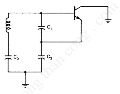
This circuit has practical advantage of being able to provide another degree of design freedom when making  $C_0$  much smaller than  $C_1$  and  $C_2$ . The  $C_0$  can be adjusted for the desired oscillating frequency  $\omega_0$ , which is determined from:
