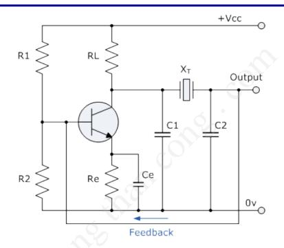
These types of crystal oscillators are designed around the CE amplifier stage of a Colpitts oscillator. The input signal to the base of the transistor is inverted at the transistors output. The output signal at the collector is then taken through a 180° phase shifting network which includes the crystal operating as an Inductor (parallel resonance area). The output is also fed back to the input which is "in-phase" with the input providing the necessary positive feedback.
