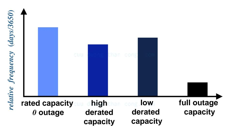
outage capacity of a generating plant (MW)
