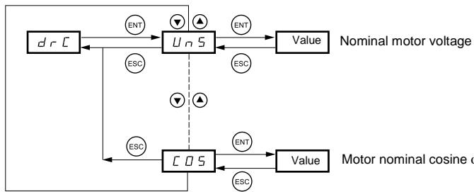
The parameters in clear boxes can only be modified when the drive is stopped and locked.
