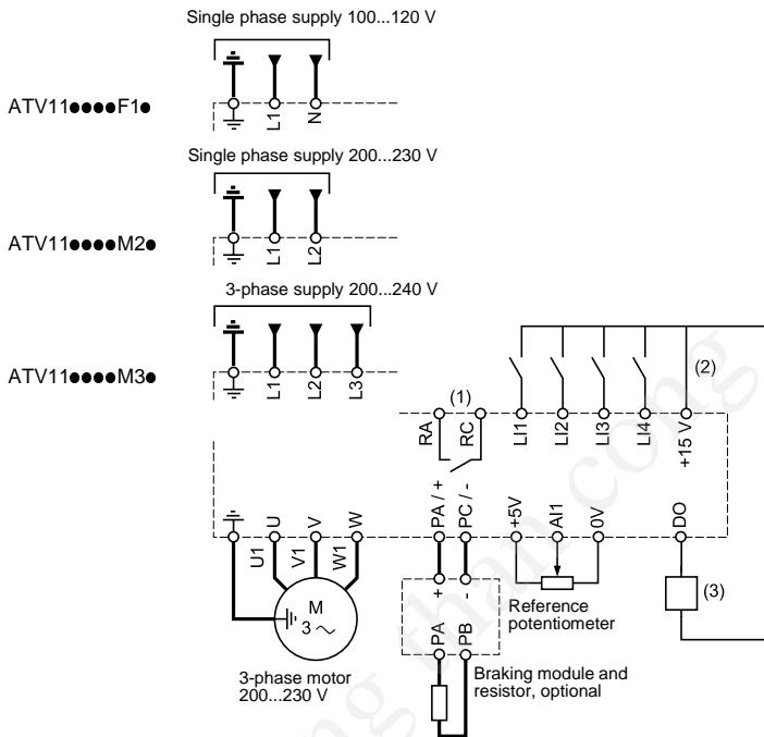
(1) Fault relay contacts, for remote indication of the drive status.
