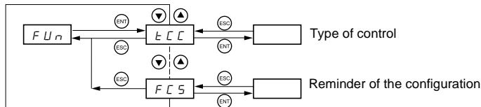
The parameters in clear boxes can only be modified when the drive is stopped and locked.
