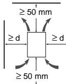
Install the unit vertically, at  $\pm 10^\circ$ .
