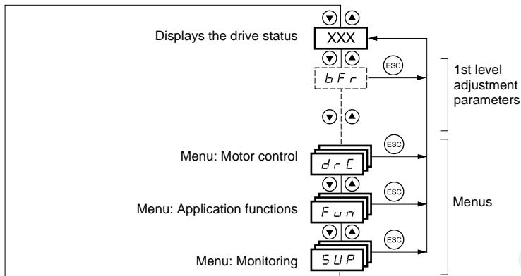
The parameters in clear boxes can only be modified when the drive is stopped and locked.
