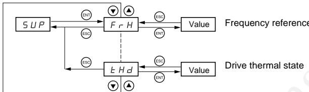
When the drive is running, the value displayed is that of one of the monitoring parameters. The default value which is displayed is the motor reference (parameter FrH).
