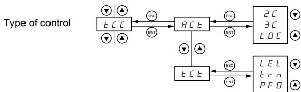
The parameters in clear boxes can only be modified when the drive is stopped and locked.
