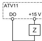
Diagram with external power supply:
