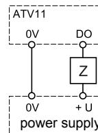
If it is a logic output: Z = low-voltage relay or input.
