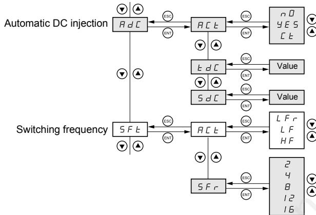
The parameters in clear boxes can only be modified when the drive is stopped and locked.
