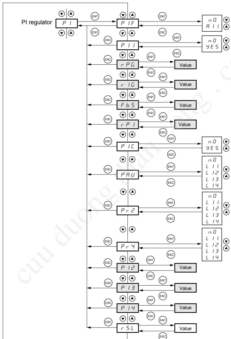
The parameters in clear boxes can only be modified when the drive is stopped and locked.
