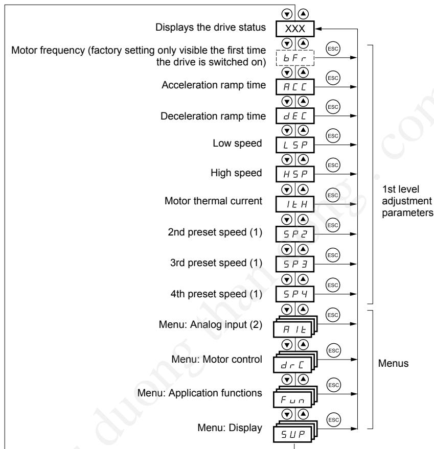
(1) The preset speeds only appear if the corresponding function has remained at the factory setting or has been reconfigured in the FUn menu.
