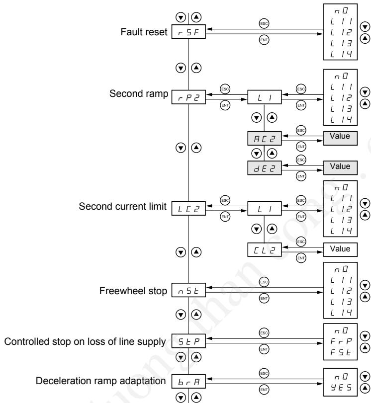
The parameters in clear boxes can only be modified when the drive is stopped and locked.
