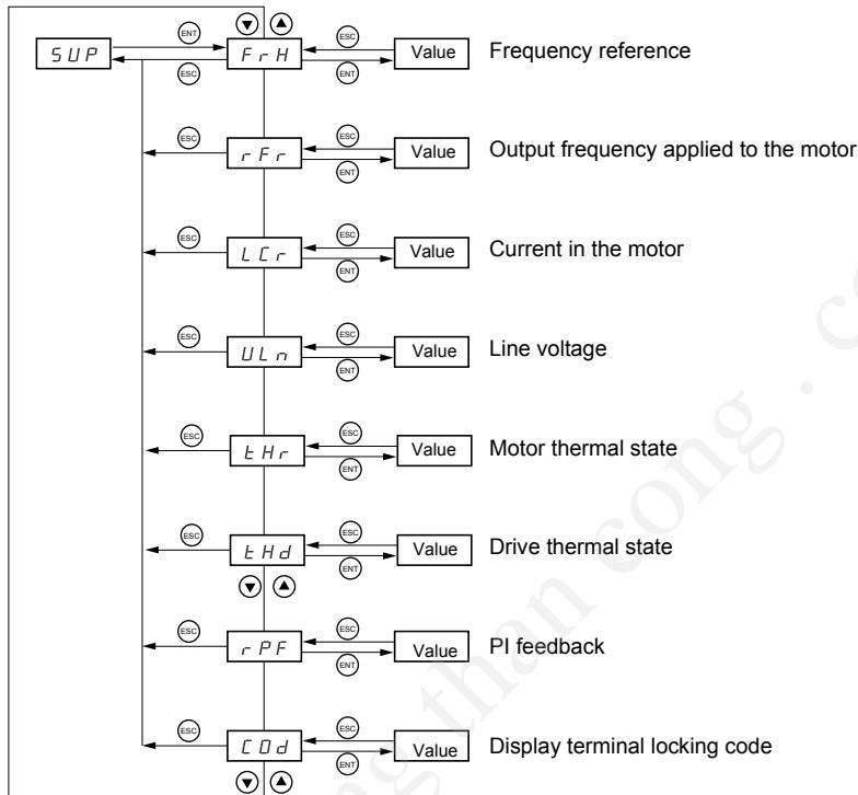
When the drive is running, the value displayed is that of one of the monitoring parameters. The default value which is displayed is the motor reference (parameter FrH).
