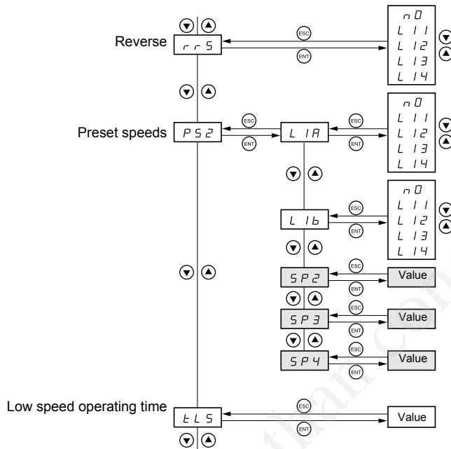
The parameters in clear boxes can only be modified when the drive is stopped and locked.
