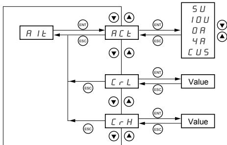
These parameters can only be modified when the drive is stopped and locked.
