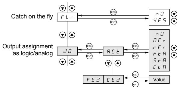
The parameters in clear boxes can only be modified when the drive is stopped and locked.
