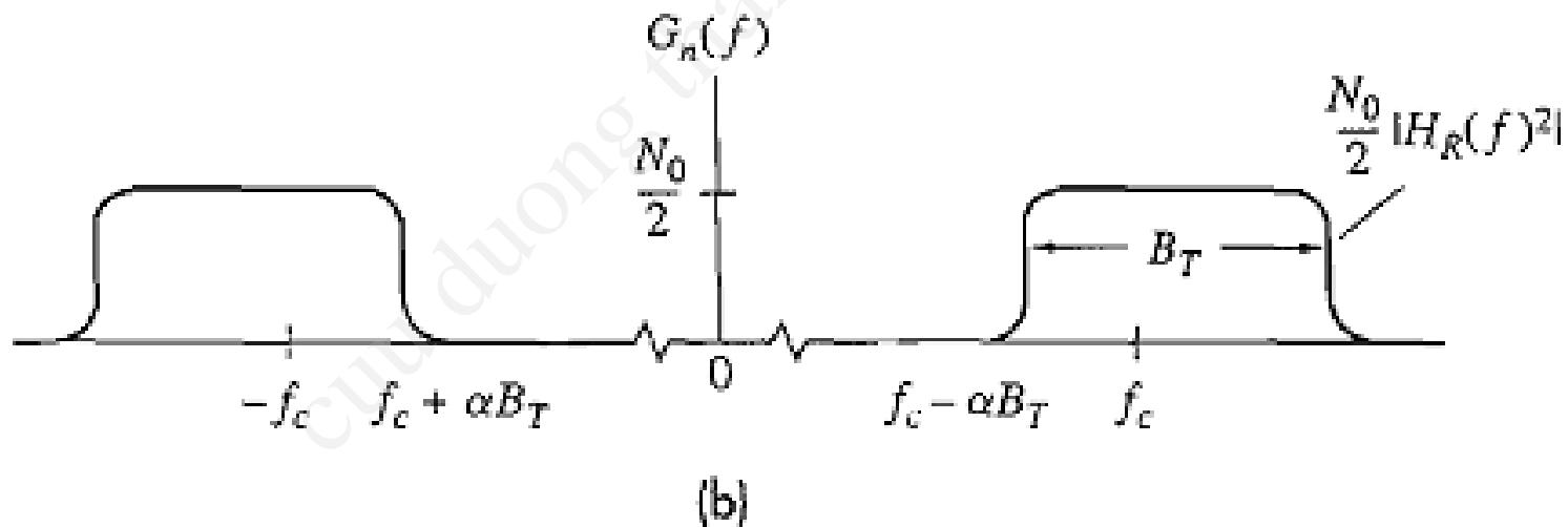
Bandpass filtered white noise. (a) Block diagram; (b) power spectrum.
