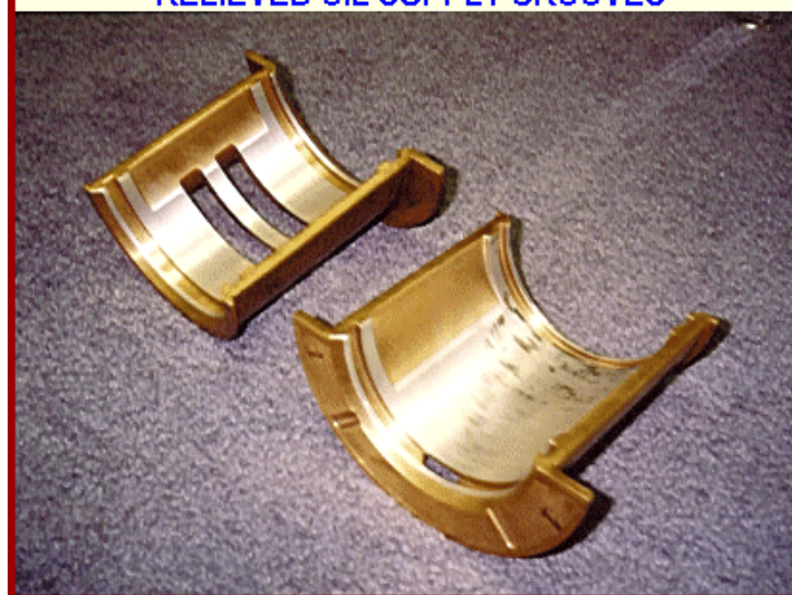
PLAIN JOURNAL BEARINGS WITH RELIEVED OIL SUPPLY GROOVES
