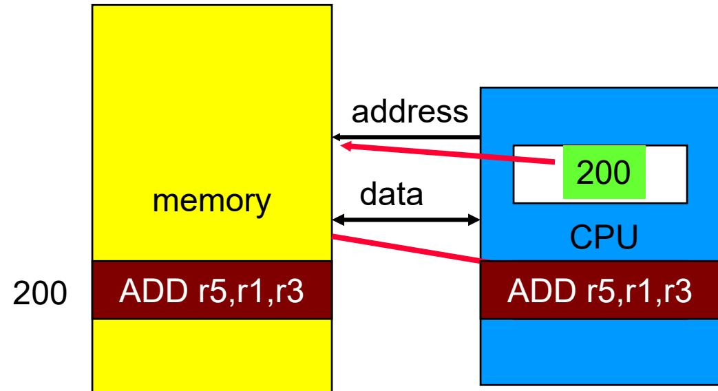
A computer whose memory holds both data and instructions is known as a ***von Neumann*** machine. The **CPU fetches** the instruction from memory, decodes the instruction, and executes it. The program counter does not directly determine what the machine does next, but only indirectly by pointing to an instruction in memory
