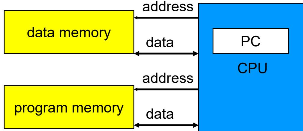
Harvard machine has separate memories for data and program. The program counter points to program memory, not data memory. As a result, it is harder to write self-modifying programs (programs that write data values, then use those values as instructions) on Harvard machines.
