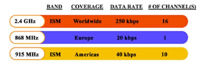
[source: Gary Legg, ZigBee: Wireless Technology for Low-Power Sensor Networks, http://www.eetimes.com/document.asp?doc\_id=1275760]
